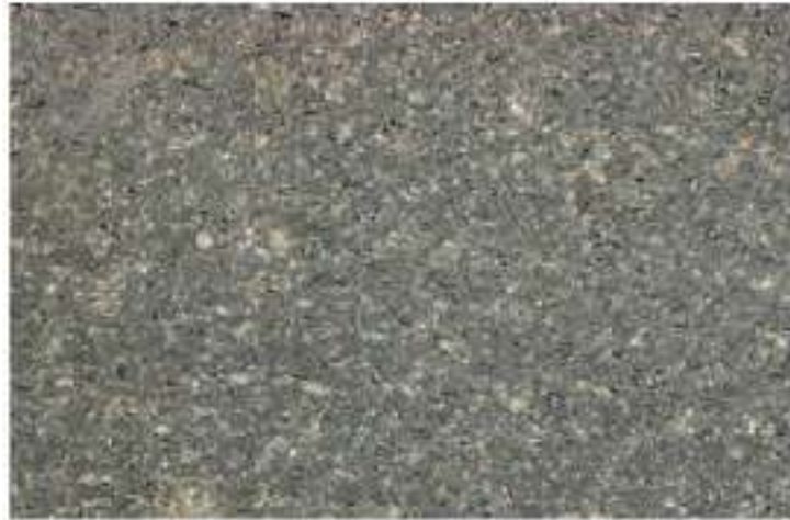
(B) An aphanitic texture consists of mineral grains too small to be seen without a microscope. The sample shown here is rhyolite. Only a few grains are large enough to be seen. Most are microscopic. Aphanitic texture results from rapid cooling.
